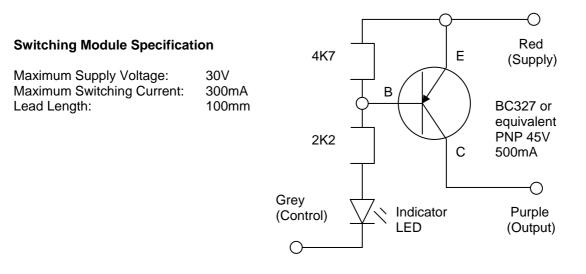
Figure 18 - Transistor Switch - Circuit Diagram
